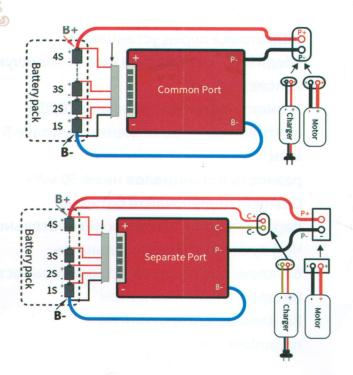
First, Preparation before installation Make sure the batteries are of good consistency. The volt difference is no more than 0.05V, inner resistance is no more than 5m $\Omega$ , capacity difference lower than 30mAh. Connect the batteries in parallel first and then in series. the better performance of batteries consistency is, the higher performance of the BMS.
